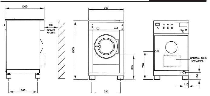
A - Ventilation Overflow Outlet, B - Soft Water Connection (cold), C - Warm Water Connection, D - Hard Water Connection (cold),
