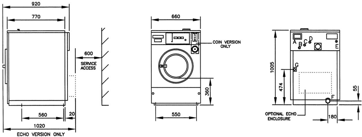
**A - Ventilation Overflow Outlet, B - Soft Water Connection (cold), C - Warm Water Connection, D - Hard Water Connection (cold), E - Electrical Connection, F - Drain Outlet, G - Steam Connection**
